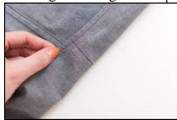
Fig (3): Flat felled seams look finished on both sides of a garment.
